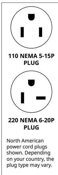
for power. These cycles can be daisy-chained together with up to 4 units per 15 A circuit. This outlet should be a NEMA 6-20R and have the same configuration as the plug. No adapter should be used with this product. Matrix daisy-chain cord adapters are sold separately.
